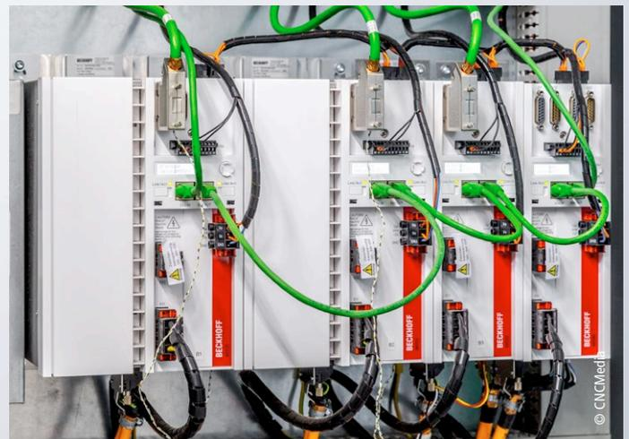
The AX5000 Servo Drives ensure dynamic and precise shaft movements of the laser head.
