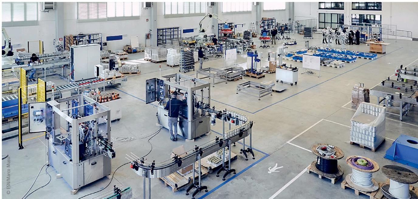
Based on a modular machine design, the ESN Group manufactures custom, end-of-line packaging solutions for a wide range of industries.
