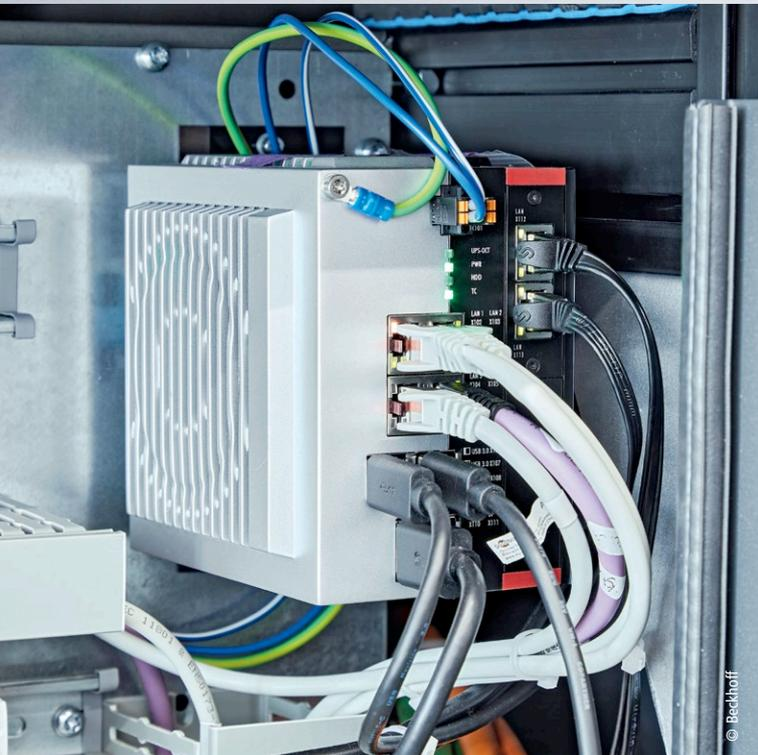
The high-performance C6032 ultra-compact Industrial PC controls all machine and process sequences with numerous TwinCAT software functions, such as TwinCAT Vision.
