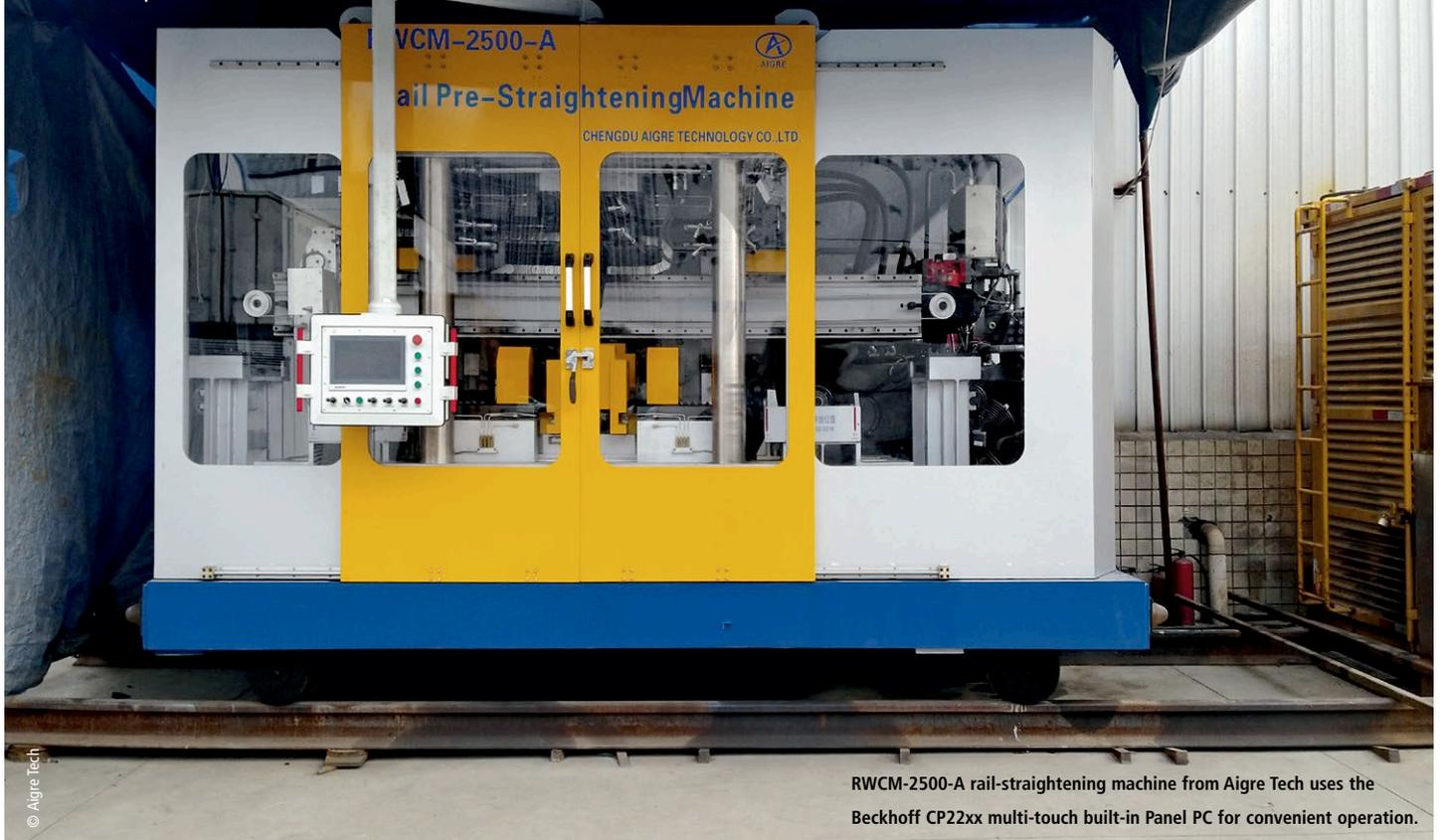
RWCM-2500-A rail-straightening machine from Aigre Tech uses the Beckhoff CP22xx multi-touch built-in Panel PC for convenient operation.
