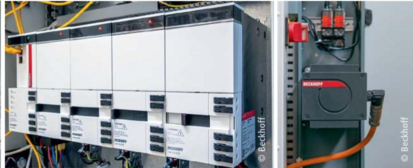
Above: The AX8000 multi-axis servo system ensures highly dynamic and precise motion control.
