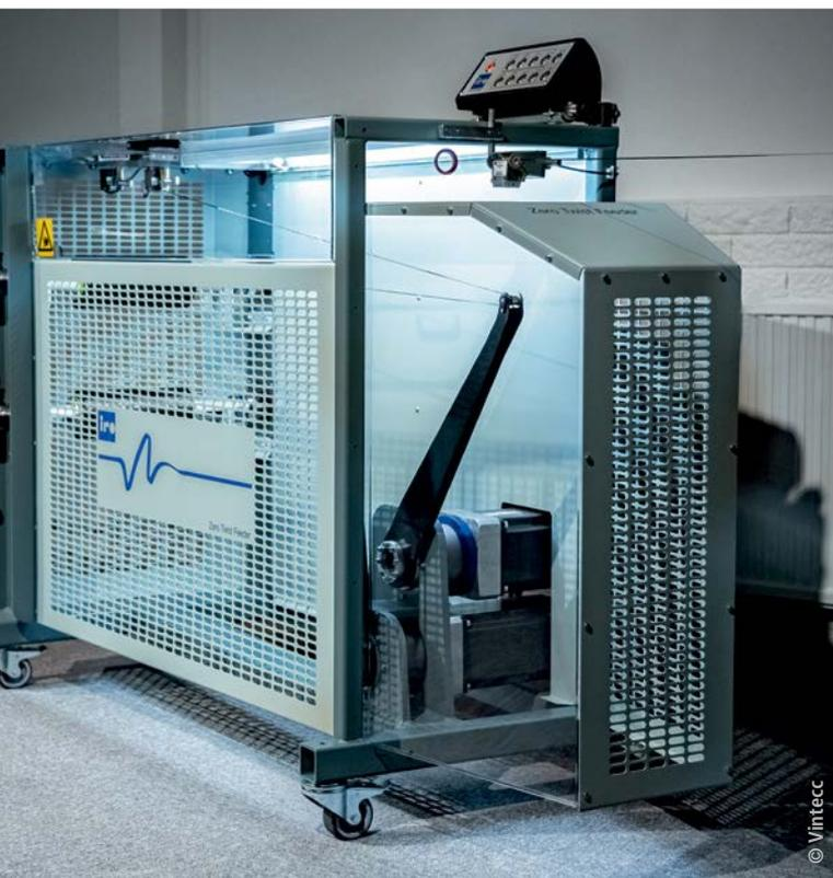
The Zero Twist Feeder delivers the yarn for the weaving process with high precision.
