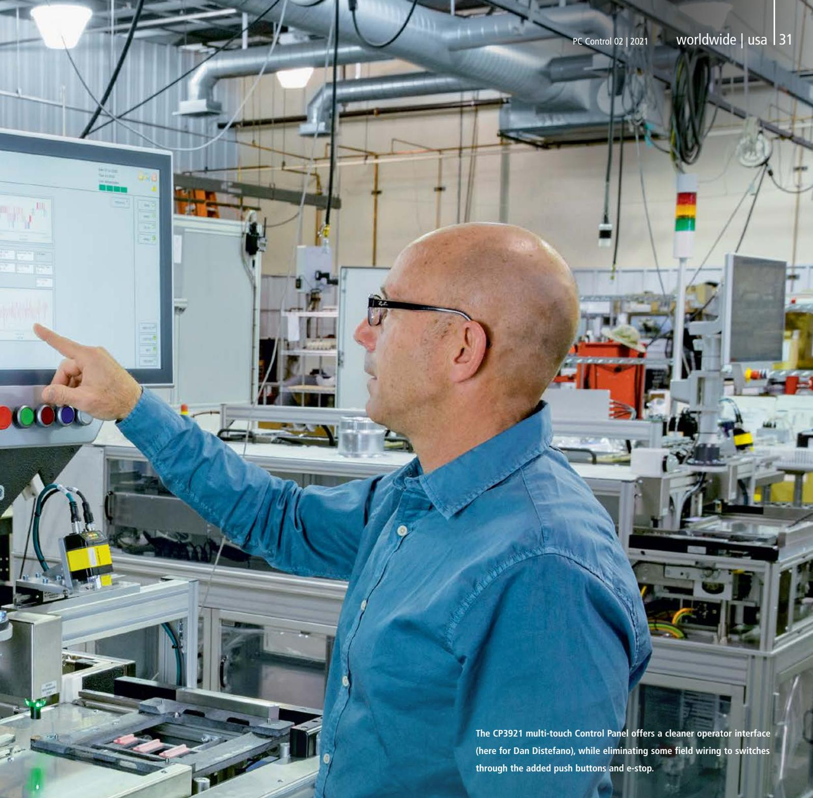
The CP3921 multi-touch Control Panel offers a cleaner operator interface (here for Dan Distefano), while eliminating some field wiring to switches through the added push buttons and e-stop.
