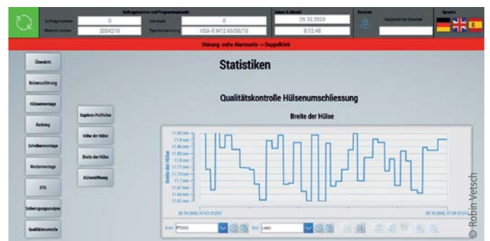
Representation of the sleeve width as one of the quality criteria for the sleeve enclosure
