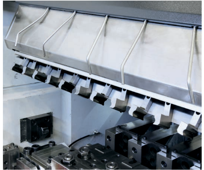
The servo-controlled gripper fingers convey the products with high precision and dynamics between the individual processing steps.
